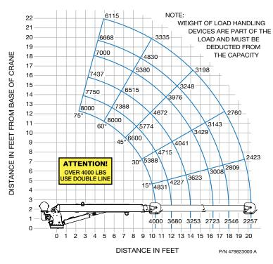
Note: Weight of load handling devices are part of the load and must be deducted from the capacity.
