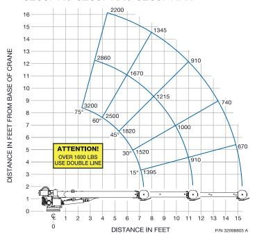
Note: Weight of load handling devices are part of the load and must be deducted from the capacity.
