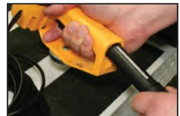
3. Attach the other end of the back-up cord to the connector currently used by the antenna on the control receiver. The control receiver is located on the back of the crane mast.
