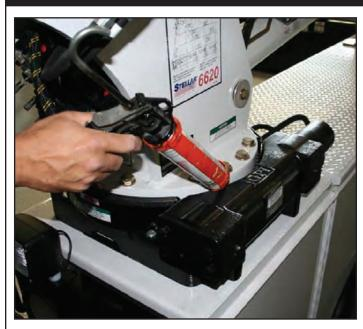
**Rotation Worm Gear and Open Gear Teeth** Use a heavy Moly Lube grease (Stellar PN 4460) to lubricate the worm gear and open gear teeth of the rotation bearing. Slowly rotate the crane while pumping the grease between the worm and rotation gear. This should be greased every month or sooner depending on the usage of the crane. Another way of applying the grease would be to remove the gear guard and brush the Molube grease between the gear teeth of the rotation bearing.
