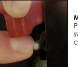
Manual Winch Down: Push the manual winch switch down to lower the cable and hook.
