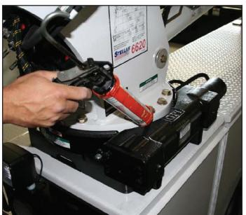
Rotation Worm Gear and Open Gear Teeth Use a heavy Moly Lube grease (Stellar PN 4460) to lubricate the worm gear and open gear teeth of the rotation bearing. Slowly rotate the crane while pumping the grease between the worm and rotation gear. This should be greased every month or sooner depending on the usage of the crane. Another way of applying the grease would be to remove the gear guard and brush the Molube grease between the gear teeth of the rotation bearing.
