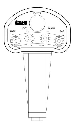
This crane is operated by a radio control system which operates an electronic valve bank. The controller (as shown) operates the following functions:
