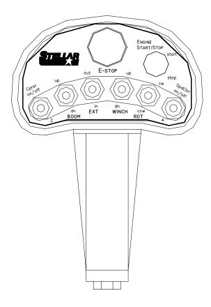
This crane is operated by a radio control system which operates an electronic valve bank. The controller (as shown) operates the following functions:
