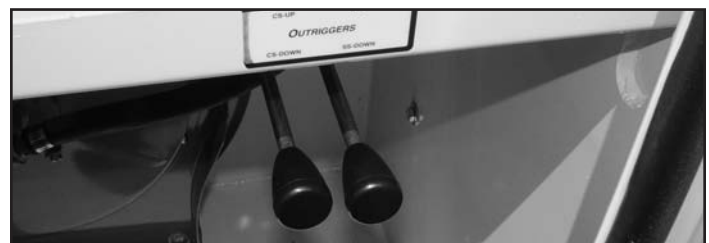
Outrigger control panel, located in the crane compartment.
