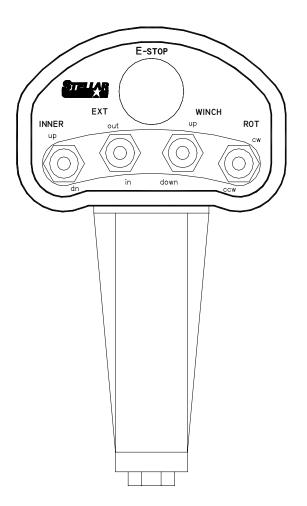
This crane is operated by a radio control system which operates an electronic valve bank. The controller (as shown) operates the following functions:
