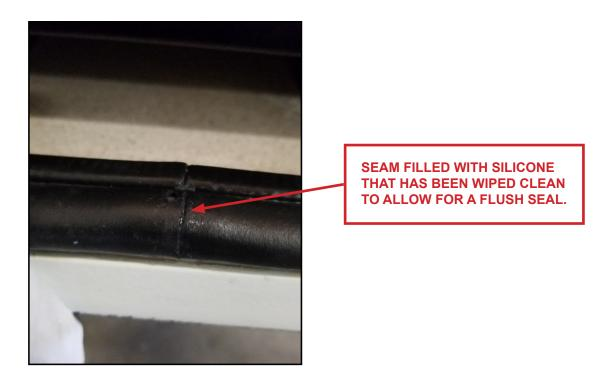
9. The door seam gasket (D-shaped seal with adhesive) must be applied to the full length of the outer door. It must be applied to the inside radius of the double bend. Before applying gasket to door, position the red tape in line with the tangent line of the radius as shown below.
