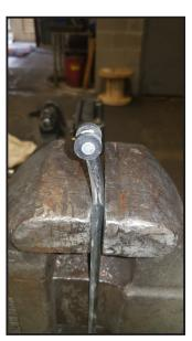
DIRECTION TO BEND ROD NECK ROLLER HEAD WHEN ORIENTED CORRECTLY.
