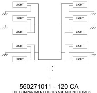
THE COMPARTMENT LIGHTS ARE MOUNTED BACK TO BACK ON THE DIVIDER PANEL BETWEEN THE FRONT AND MID COMPARTMENT AS WELL AS THE HORIZONTAL AND REAR COMPARTMENTS. THE OTHER LIGHT IS MOUNTED ON THE DIVIDER PANEL BETWEEN THE TWO FRONT COMPARTMENTS FACING THE CAB.
