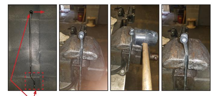
DIRECTION TO BEND ROD NECK ROLLER HEAD WHEN ORIENTED CORRECTLY.
