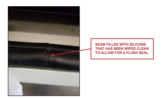
9. The door seam gasket (D-shaped seal with adhesive) must be applied to the full length of the outer door. It must be applied to the inside radius of the double bend. Before applying gasket to door, position the red tape in line with the tangent line of the radius as shown below.
