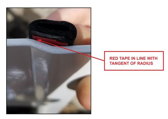
10. Cut door seam gasket to full length of door and apply flush. Firmly press gasket into door to make sure adhesive holds
