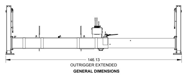
EXTENSION STROKE = 54.00in UP/DOWN LEG STROKE = 27.00in
