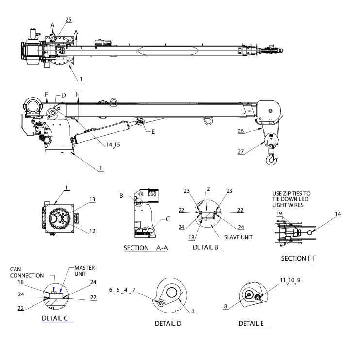
NOTES: 1. APPLY LOCTITE 242 TO THREADS BEFORE INSTALLATION
