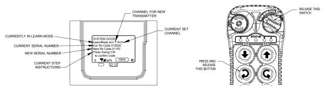
Figure 3—LCD screen display & transmitter during step 3
