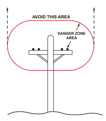
1. Do not place any part of the crane or load inside the Danger Zone.
