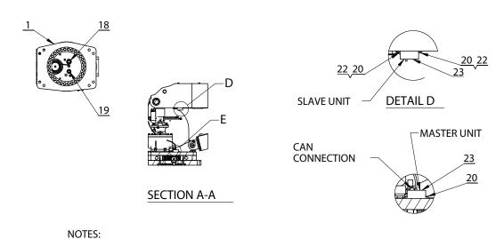
APPLY LOCTITE 242 TO THREADS BEFORE INSTALLATION
