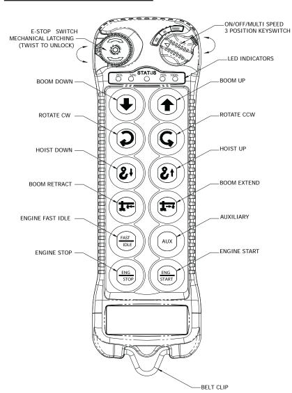
**E-stop Switch**—Push to activated, Twist to release. Shuts down all outputs from receiver.
