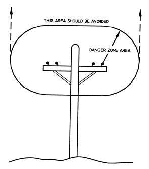
1. Cranes shall be operated so that no part of the crane or load enters into the danger zone shown above.
