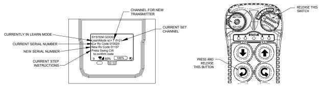
Figure 3—LCD screen display & transmitter during step 3
