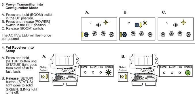
NOTE: If left idle in SETUP mode for over 30 seconds, the receiver will time out. The (LINK) light and (STATUS) light will flash RED rapidly. To return to SETUP mode, repeat step 4.
