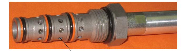
VERIFY MOVEMENT IN PORTS WHILE MANUALLY OVER-RIDING CARTRIDGE.
