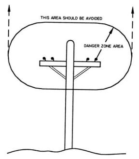
1. Cranes shall be operated so that no part of the crane or load enters into the danger zone shown above.
