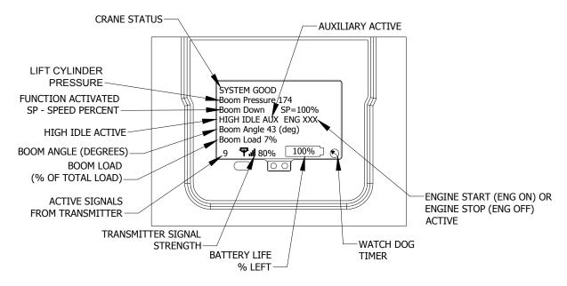
**CRANE STATUS**—shows current status of the crane. If any alarms are occurring they will be displayed here. Otherwise, it will say system good. **Note: Reference Troubleshooting section for alarm descriptions.**
