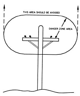
Cranes shall be operated so that no part of the crane or load enters into the danger zone shown above.
