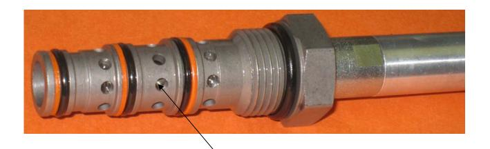
VERIFY MOVEMENT IN PORTS WHILE MANUALLY OVER-RIDING CARTRIDGE.
