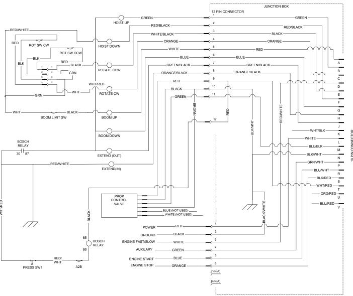
19 PIN CONNECTOR REFRENCE 680040 FOR PENDANT SCHEMATIC
