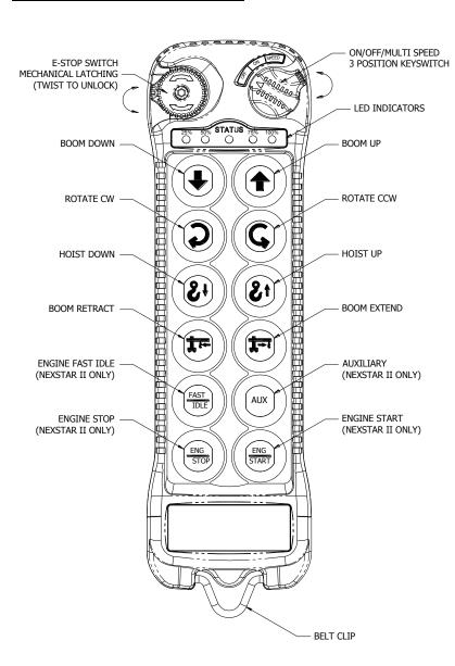
**E-stop Switch**—Push to activated, Twist to release. Shuts down all outputs from receiver.
