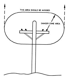
Cranes shall be operated so that no part of the crane or load enters into the danger zone shown above.
