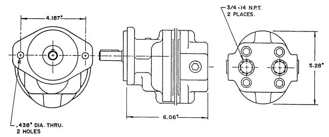
Adapter: SAE "A" 2 bolt flange (direct mount only). Shaft: Straight shaft key 3/4 dia. x 2 3/4 long. 3/16 sq. key x 1 5/8 long.
