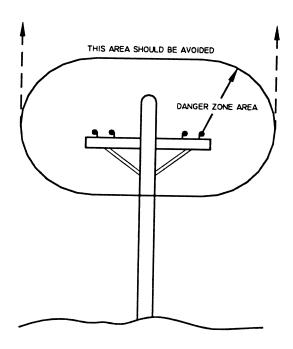
22 Cranes shall be operated so that no part of the crane or load enters into the danger zone shown above.
