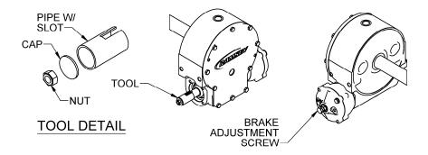
After welding the cap and nut to the tubing, slot the tubing as shown. This will allow the special adapter to slide over the keyway and then act as a large socket. A torque wrench can then be used to apply the proper torque. Turn the torque wrench so that the drum turns in the spool out direction or lowering direction. The torque ratings should be between 15-18 ft-lbs.
