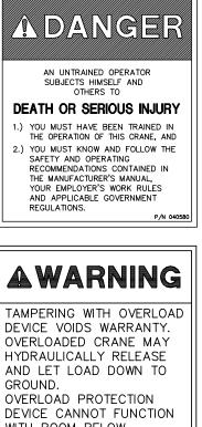
DEVICE CANNOT FUNCTION WITH BOOM BELOW HORIZONTAL (0°). HOIST UP, BOOM DOWN, AND EXTEND OUT WILL BE INOPERATIVE WHEN CRANE IS IN OVERLOAD CONDITION. P/N 040632
