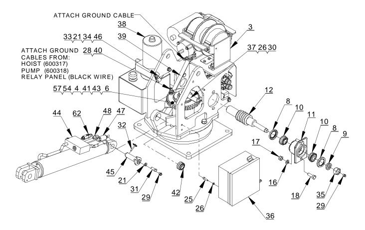
HYDRAULICS: PORT A-1 RETRACT PORT A-2 BOOM DOWN PORT A-3 CCW BOTTOM MOTOR PORT PORT B-1 EXTEND PORT B-2 BOOM UP PORT B-3 CW TOP MOTOR PORT
