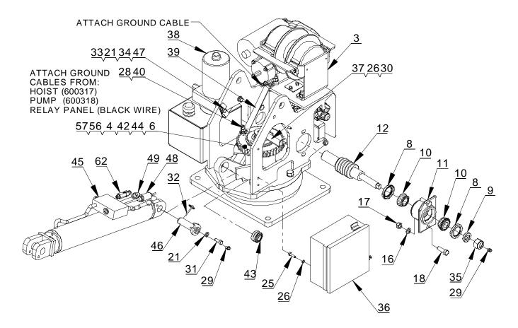
HYDRAULICS: PORT A-1 BOOM UP PORT A-2 CCW BOTTOM MOTOR PORT PORT B-1 BOOM DOWN PORT B-2 CW TOP MOTOR PORT
