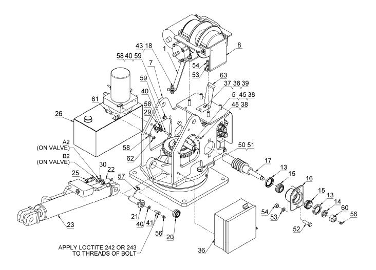
HYDRAULICS: PORT A-1 RETRACT PORT A-2 BOOM DOWN PORT A-3 CCW BOTTOM MOTOR PORT PORT B-1 EXTEND PORT B-2 BOOM UP PORT B-3 CW TOP MOTOR PORT
