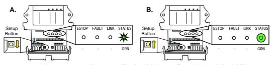
**NOTE:** If left idle in Setup Mode for over 30 seconds, the receiver will time out. The (Link) light and (Status) light will flash RED rapidly. To return to Setup Mode, repeat step 4.
