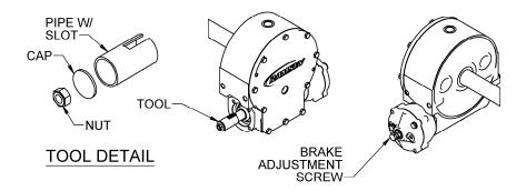
After welding the cap and nut to the tubing, slot the tubing as shown. This will allow the special adapter to slide over the keyway and then act as a large socket. A torque wrench can then be used to apply the proper torque. Turn the torque wrench so that the drum turns in the spool out direction or lowering direction. The torque ratings should be between 12-16 ft-lbs.
