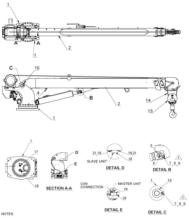
APPLY LOCTITE 242 TO THREADS BEFORE INSTALLATION
