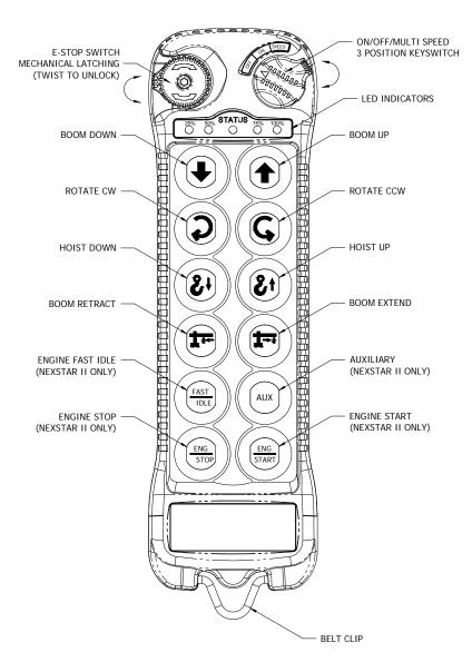
**E-stop Switch**—Push to activated, Twist to release. Shuts down all outputs from receiver.
