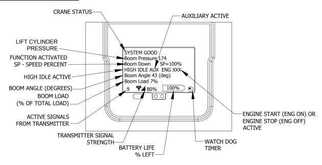
**CRANE STATUS**—shows current status of the crane. If any alarms are occurring they will be displayed here. Otherwise, it will say system good. **Note: Reference Troubleshooting section for alarm descriptions.**
