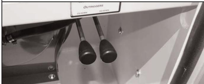
*Outrigger control panel, located in the crane compartment.*
