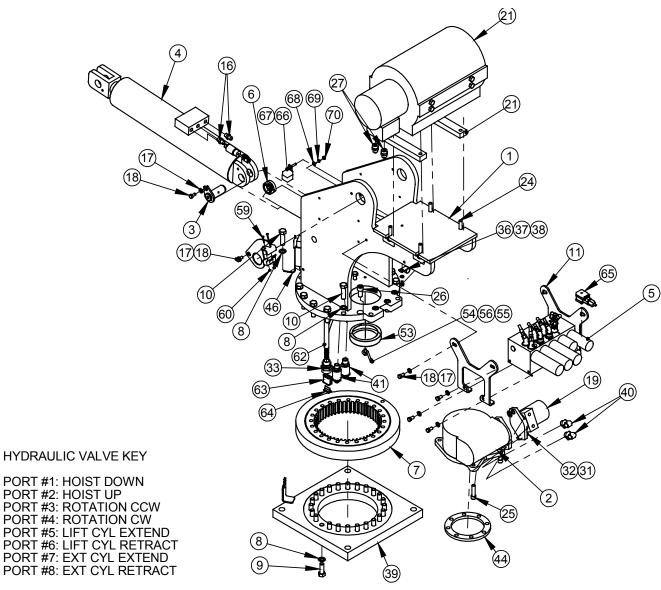
CYLINDER SEAL KIT: 366342001 COUNTER BALANCE CARTRIDGE" 480188000
